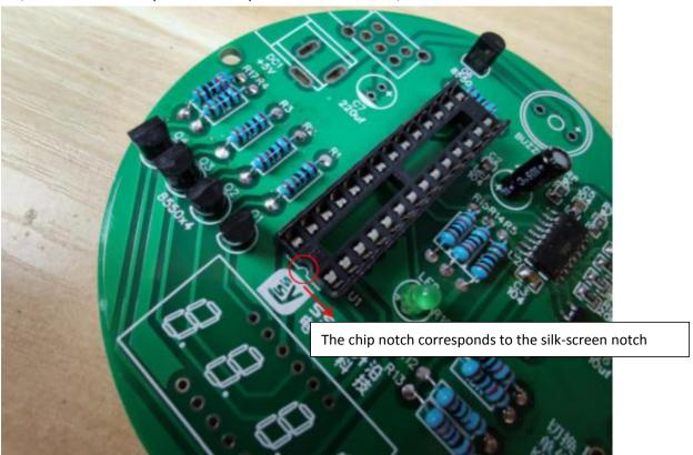
4: For welding other devices, the direction of the digital tube must be correct and not reversed;
